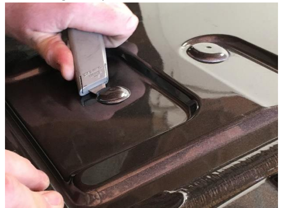
Figure 14: Roof Rack Mounting Point Plug Removal
