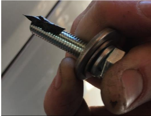
Figure 16: Silicone Sealant Applied to the M8 Mounting Hardware
